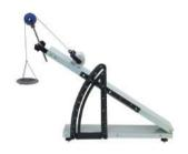
This versatile and tough steel inclined plane includes a graduated protractor and an adjustable pulley. Incline is 4" wide x 23" long. Includes a 14 oz.
